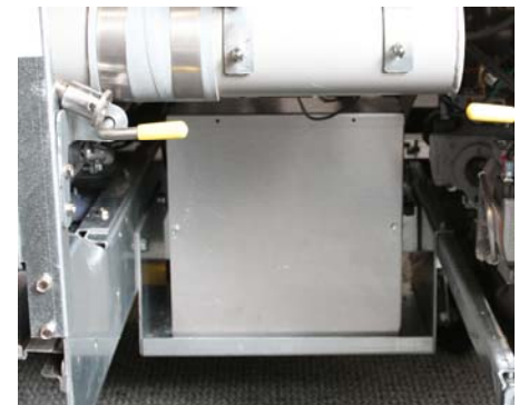
Figure 2: The ATO box is shown in the JIB cabinet. Remove the screws securing its shelf and lower to the floor to ease access for positioning the plumbing assembly.
